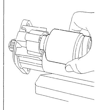
Disassembling solenoid switch
